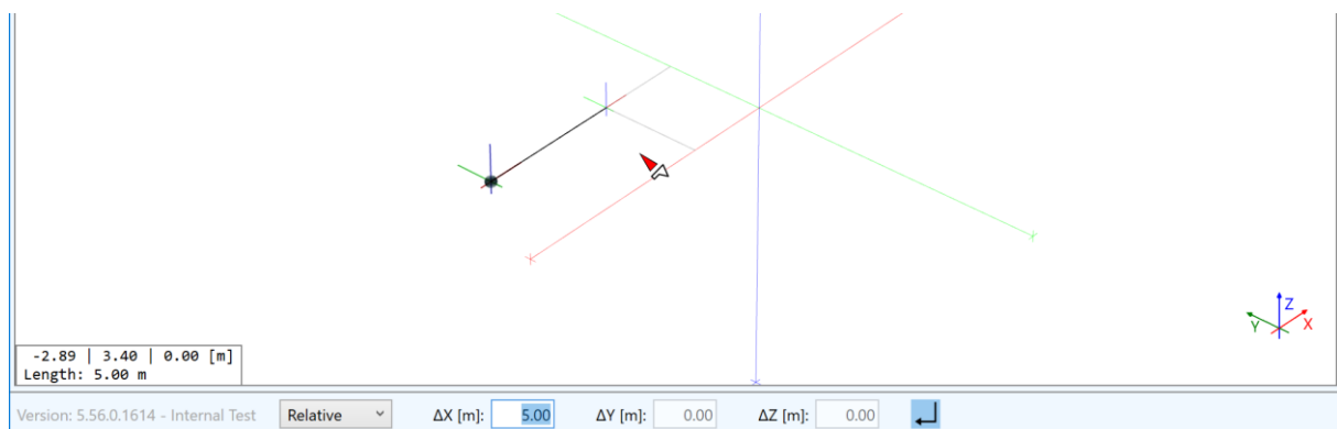
Figure 6.14 Coordinate entry relative to reference point - in this case by using the X-constraint and a distance of 5 m from the reference point.
