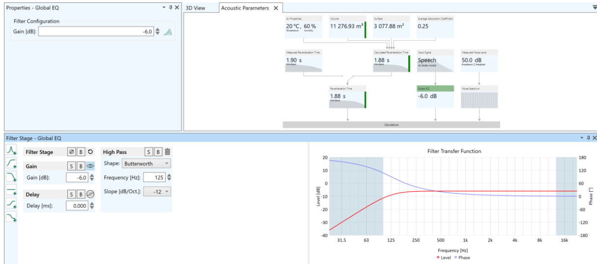
Figure 5.23 The global EQ allows applying signal processing to the entire sound system. In the example shown, a gain of -6 dB is applied as well as a light high-pass filter.
