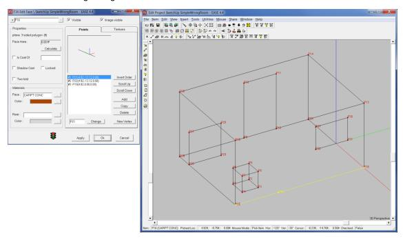
A border of the model is highlighted in yellow and the properties dialog is open for the face with the problem. Even though this item looks like an *Edge*, it is actually defined as a *Face*. The *Face* has no surface area, causing the problem. Click **OK** to close the **Properties** window and use the Delete key.
