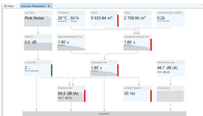
Figure 7.32 Room volume and related indicators are red due to missing or inverted faces.
