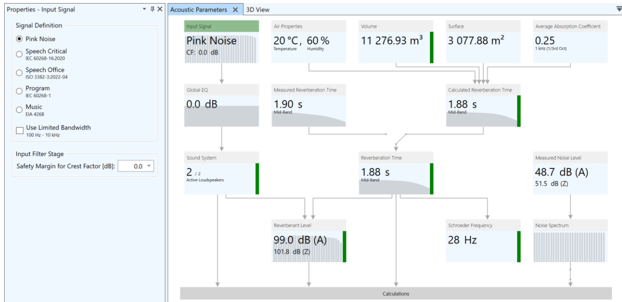
Figure 5.21 Selection of input signal with available options in the properties window on the left: pink noise, speech, program, music.
