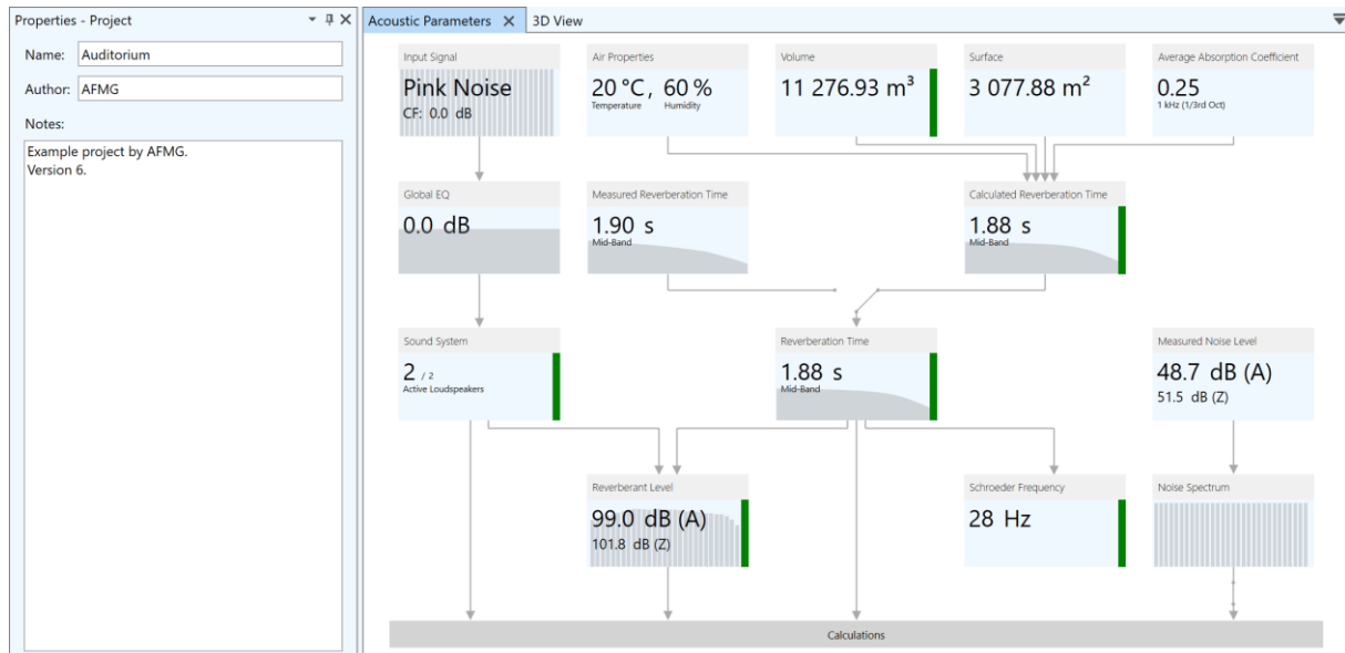
Figure 5.14 Acoustic parameters window showing various elementary properties of the room.
