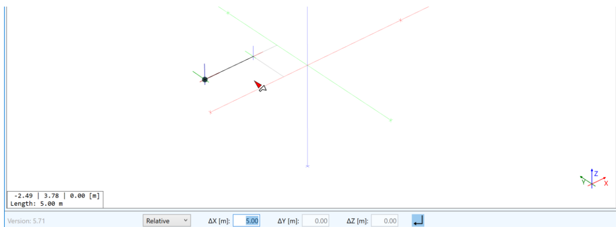
Figure 6.14 Coordinate entry relative to reference point - in this case by using the X-constraint and a distance of 5 m from the reference point.
